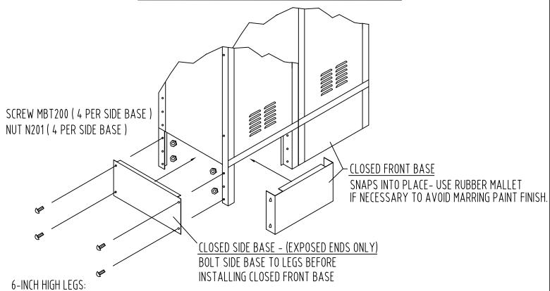
LEGS ARE STANDARD AND ARE INTEGRAL WITH FRAME UPRIGHTS IN FRONT REAR LEGS ARE BOLTED TO SIDE AND BACK (USE TWO REAR LEGS FOR 1-WIDE AND 3-WIDE UNITS).
